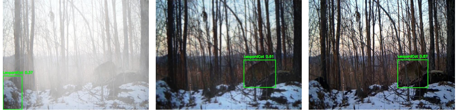
Fig 8. YOLOv11 animal detection on hazy image, dehazed image and ground truth respectively.
